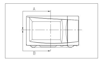
NOTE: A small gap may be acceptable if the microwave leakage does not exceed 4mW/cm<sup>2</sup>.
